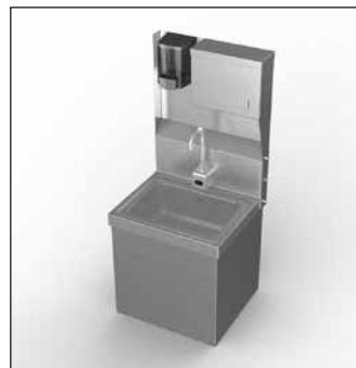
Model HSTAE $3,152 Hand Sink, wall mount, 14" wide x 10" front-to-back x 5" deep, s/s construction, 8" splash on back, wall brackets, electronic splash mount faucet, lever waste, overflow, P-trap, soap & towel dispenser, apron, NSF
