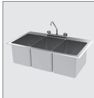
DIHS-3-1014 $1,490 Drop in sink 3 compartment 10" wide x 14" front to back x 10" deep 32 x 18.5 over flange, with 2 4"OC faucet holes 18ga 300 series s/s construction, with faucet & basket strainer. NSF
