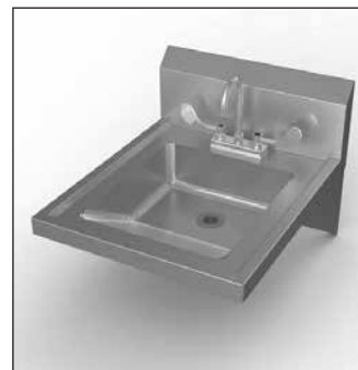
Model HSADA-D $1,685 Wall mount ADA Hand Washing Sink, 18GA 300 series, s/s, Box Marine Dripless Edge Bowl, 16 x 14 , 8" splash on rear. Faucet holes 4" on center. Deck mounted faucet, wrist handles. Basket drain and Z bar included, NSF. For electronic faucet see hand sink accessories
