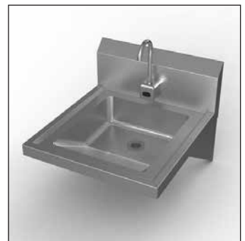
Model HSADA-SE $3,148 Wall mount ADA Hand Washing Sink, 18GA 300 series, s/s, Box Marine Dripless Edge Bowl, 16 x 14, 8" splash on rear. Faucet holes 4" on center. Splash mounted faucet, wrist handles. Basket drain and Z bar included, NSF. For electronic faucet see hand sink accessories.
