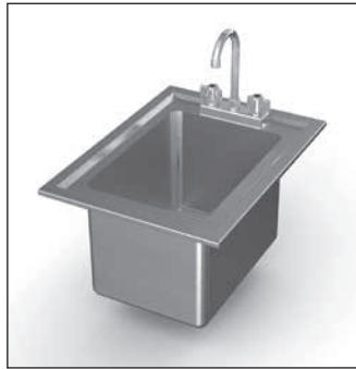
Model DIHS-1-10 $521 Drop In Sink, 1 compartment, 10" wide x 14" front/back x 10" deep, 14 1/2" x 19 3/4" over flange, with 4" O.C. faucet holes, 18 gauge 300 series s/s construction, with faucet & basket strainer, NSF
