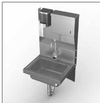
Model HSDTE $2,923 Hand Sink, wall mount, 14" wide x 10" front-to-back x 5" deep, s/s construction, 8" splash on back, wall brackets, electronic splash mount faucet, lever waste, overflow, P-trap, soap & towel dispenser, NSF
