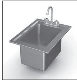
Model DIHS-1-2116 $721 Drop in sink 1 compartment 21" wide x 16" front to back x 8" deep 23 x 20.5 over flange, with 4"OC faucet holes 18ga 300 series s/s construction, with faucet & basket strainer. NSF
