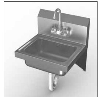
Model HSD $663 Hand Sink, wall mount, 14" wide x 10" front-to-back x 5" deep, s/s construction, 8" splash on back, wall brackets, goose-neck splash mount faucet, P-trap, overflow, NSF
